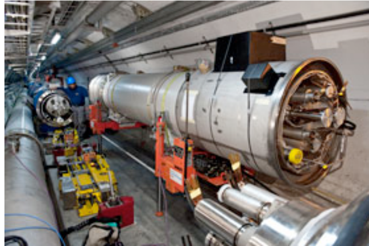
Superconducting magnets at the LHC, CERN produce a field of 6.7 T
