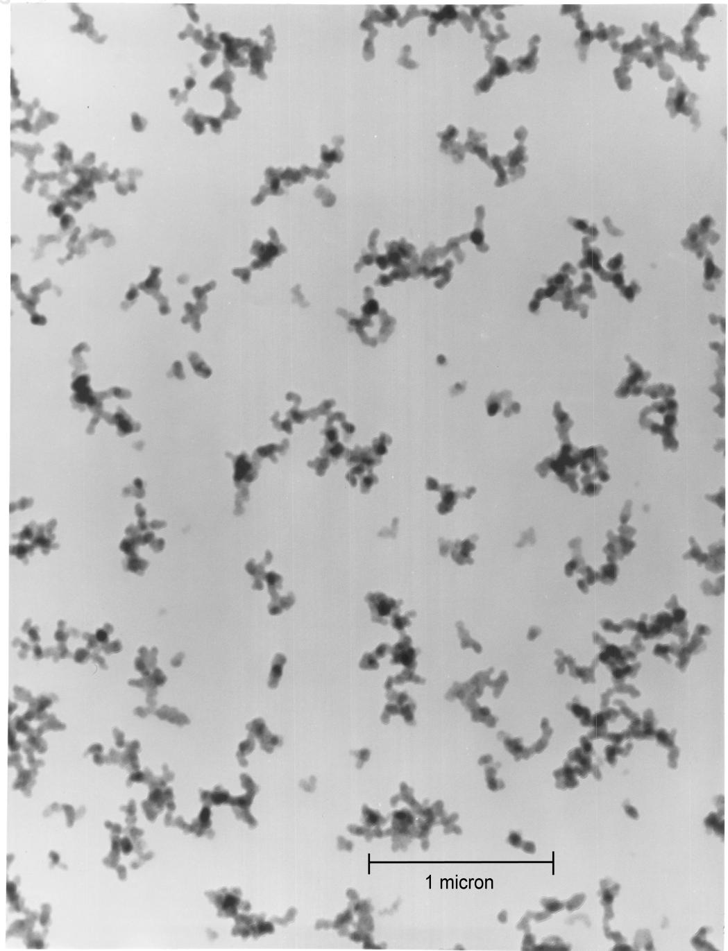
Pictures of soot taken from early in a flame (upper picture) and later in the flame (lower) after the particles grew some more.
